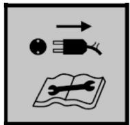
Switch off and remove plug from mains before adjusting, cleaning or if the cord is entangled or damaged
